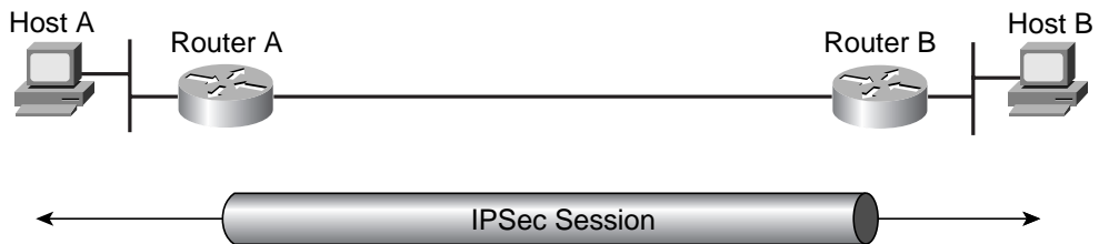
Figure 1-27 Step 4: IPsec Data Transfer
